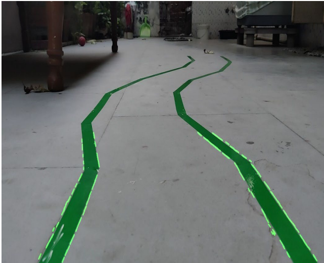
Fig. 8. Line Segment Disclosure through Probabilistic Hough Line Transformation
