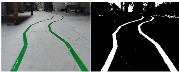
Input Webcam Feed Color Masked Image Fig. 5. Input and Color Masked Image Side by side
