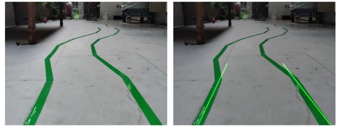
Fig. 9. Webcam Feed (left) and Lane Line Detected Image (right)
